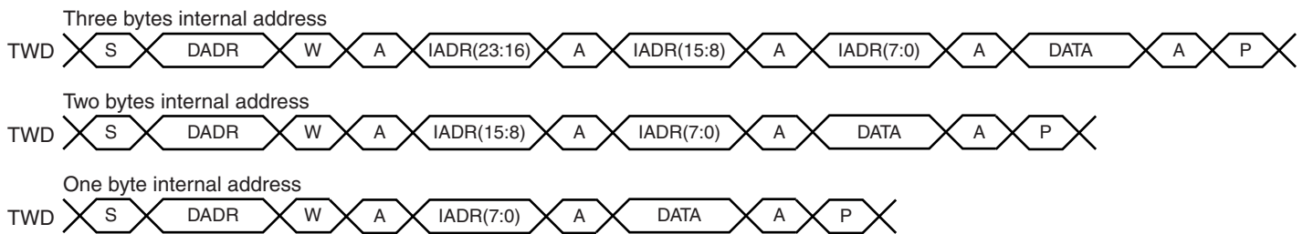
Figure 32-11. Master Write with One, Two or Three Bytes Internal Address and One Data Byte
